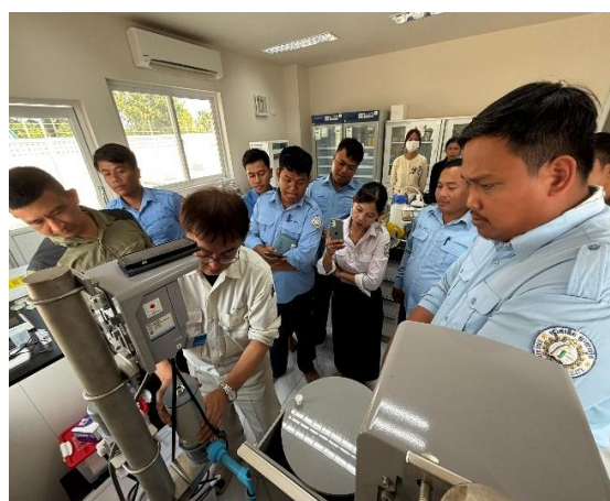
Removal of the residual chlorine meter electrode
