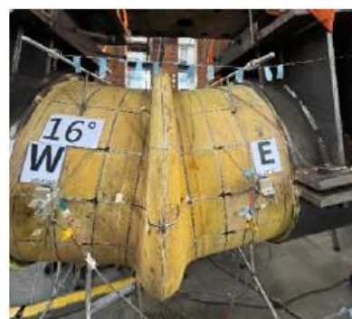
図 5-21 SPF bending test performed by the NCREE 35)
