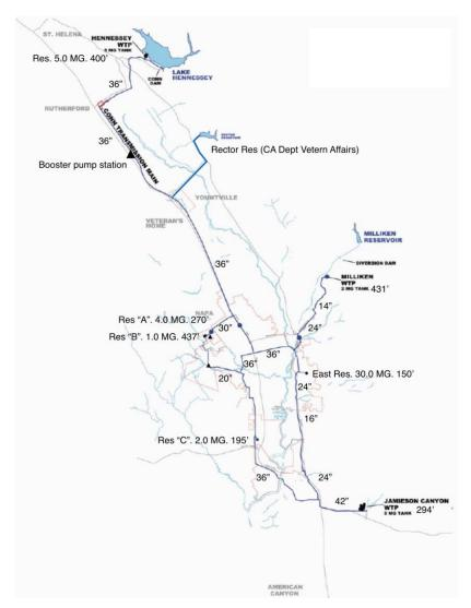
Figure 1. Napa Water System Major Pipelines and Location of Water Treatment Plants
