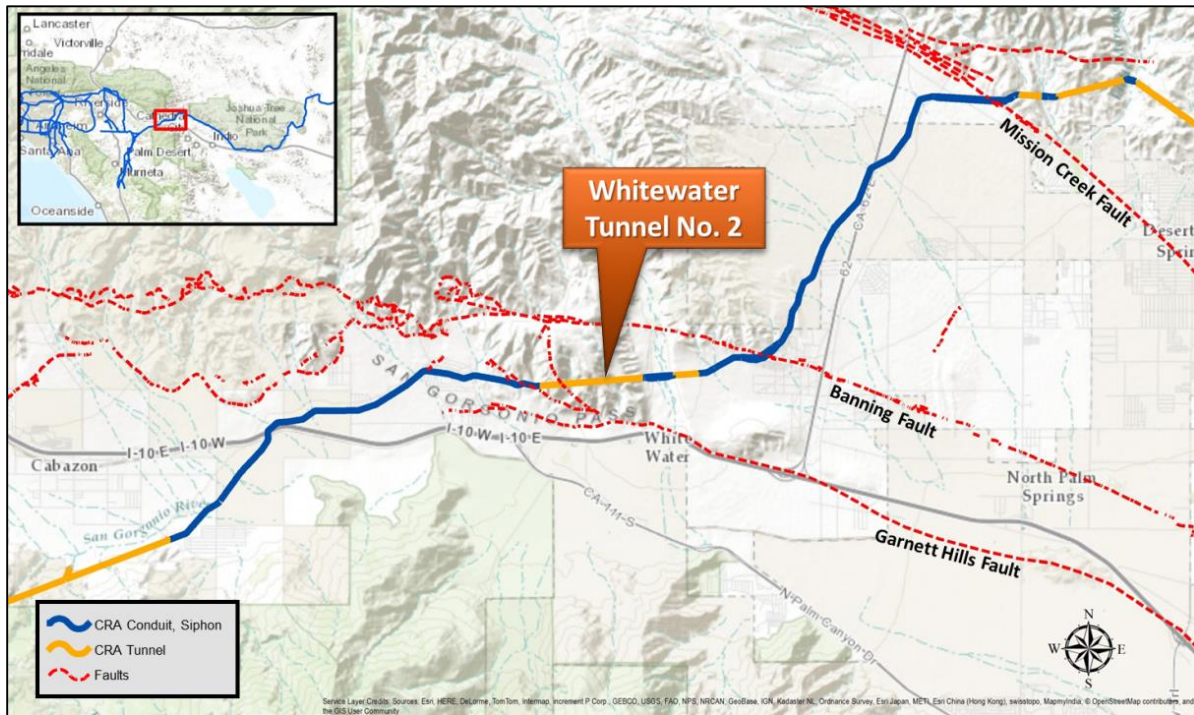
Figure 8: CRA Southern San Andreas Fault System Crossings in the San Geronio Pass
