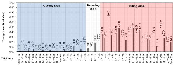
Figure 4 Damage ratio by the thickness of cutting and filling
