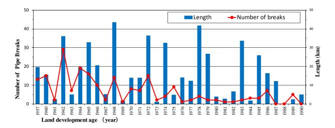
· After 1990, damaged pipeline was not found in filling area. Figure 6 Number of Pipe Breaks and Length in filling area
