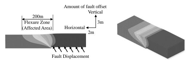
Figure 11 Distribution of Fault Displacement (Ground Deformation Analysis)
