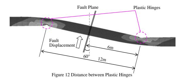
In addition, the required number of the WAVE was set as 2 WAVEs per a SPF on each plastic hinge, from the results of axial compression displacement and bending displacement.
