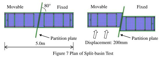
The diameter of the test pipe was 100mm (O.D.114.3mm, thickness 2.3mm, length 6m), in the assumption of one tenth model of 1000mm. As shown in Figure 8, the distance between 2 WAVEs was 600mm across the fault plane, according to FE analysis result. The test pipe was fixed in rotation direction and free in axial direction. Moreover, the amount of displacement was set as 200mm, as the result, the inner pipe wall contact angle was 18.5 degrees.
