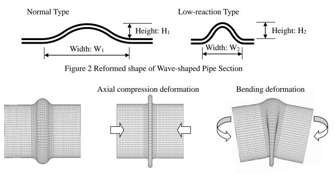
Figure 3 Deformation of Low-reaction Type of SPF
