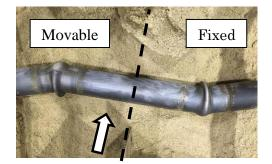
Figure 10 Test Pipe after Deformation
