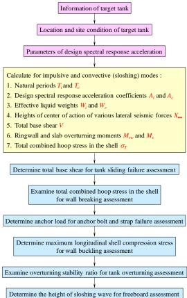
Fig. 1 Seismic assessment procedure for steel liquid storage tanks following API 650, App. E requirements.
